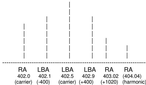
This is how the two different beacons would appear as you tuned across the band from 402 to 404.5 kHz.
