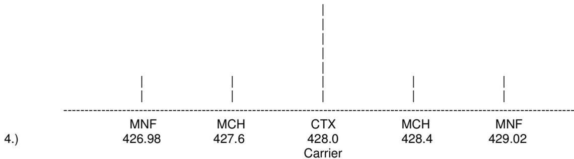
This was how the three beacons would have appeared as you tuned across the band from 426 to 430 kHz.
